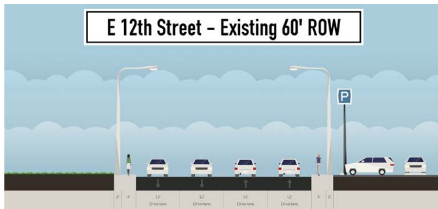
FIGURE 2-19. EXAMPLE OF EXISTING CROSS SECTIONS
